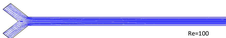
Fig.5. Flow velocity profile of a simple y-type micromixer at Re=100 .
