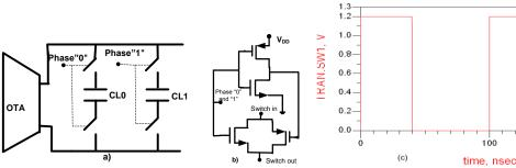
Figure 6. a) Gm-C integrator b) MOS switch scheme c) Phase "0" control signal for 1Mb/s and 10Mpulse/s
