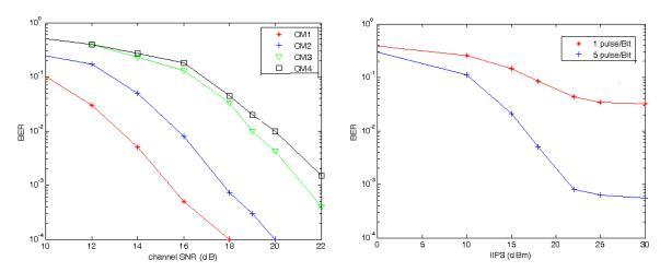
Figure 4. Channel effect on BER of ED receiver for 5pulse/Bit. Figure 5. The effect of Non-linear coefficient on BER.
