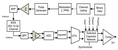
Figure 1. Transceiver architecture based on energy detection.
