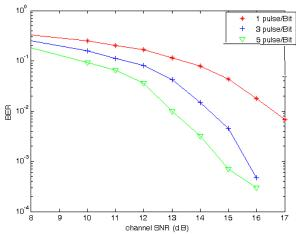
Figure 3. The effect of the number of pulse per bit on receiver performance for CM1 channel model.
