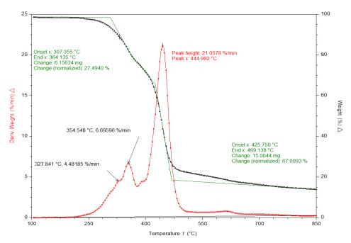
**Fig. 6.** The output curve from the TGA device software for the 50% PET and 50% Bagasse mixture with a heating rate of 20°C/min
