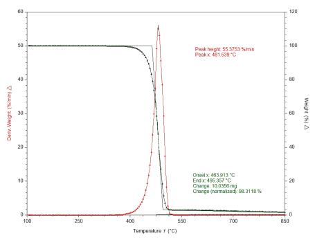
Fig. 1. Output curve from the TGA device software for LDPE at a heating rate of 20°C/min.
