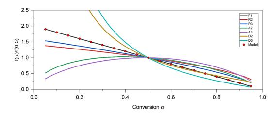
Fig. 4. Comparative curve with other models for PET.
