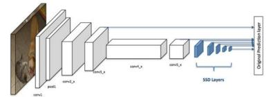
Figure 3. Architecture of a convolutional neural network with an SSD detector
