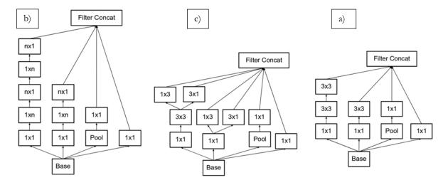
**Figure 4. a)** Resizing convolutions **b)** Converting n×n filters to a combination of 1×n and n×n filters **c)** Initial modules in which each 5×5 convolution is replaced by two 3 × 3 convolution [5]
