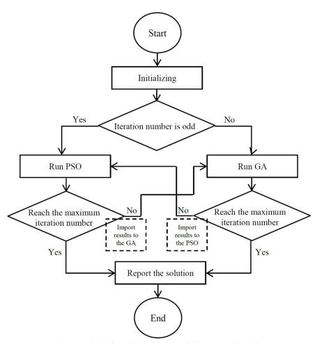
Figure 2. The flowchart of the parallel GA-PSO algorithm
