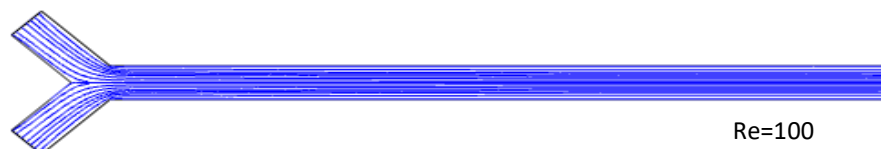
Fig.5. Flow velocity profile of a simple y-type micromixer at Re=100 .
